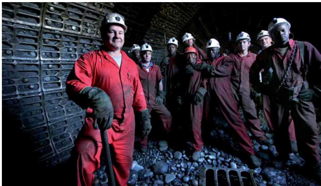
Crew replacing liners inside mill at Beatrix
